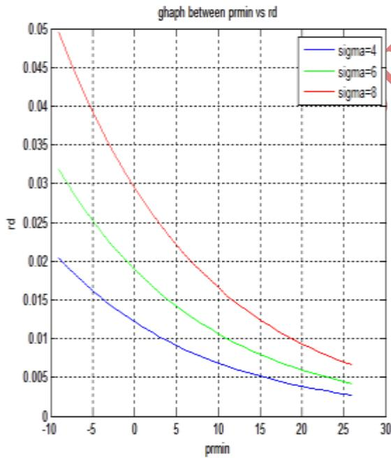
Fig.3 Graph between prmin and rd under varying shadowing effects.
