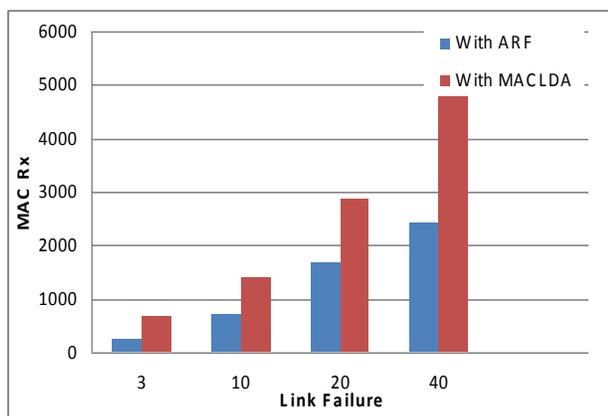
Loss recovery at MAC improved with the help of increase in MAC retransmission. This results in increase in throughput.
