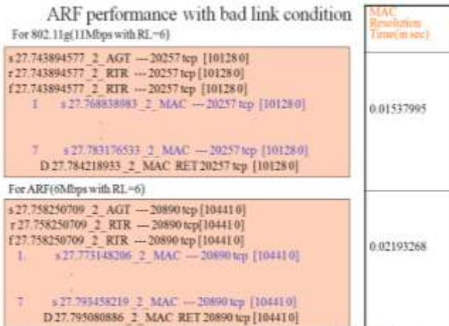
Time for MAC resolution is high in ARF in comparison with 802.11g, when wireless link is not connected which in turn reduces MAC retransmissions even in the presence of high error.
