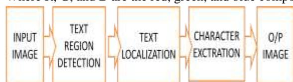
Figure 3. Basic Block diagram for edge based text extraction
