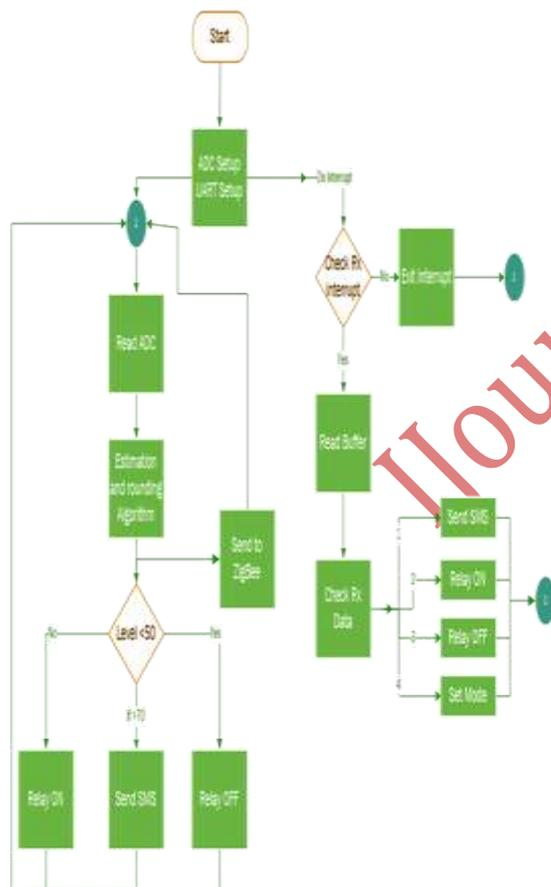
Fig. 6: System flow diagram.
