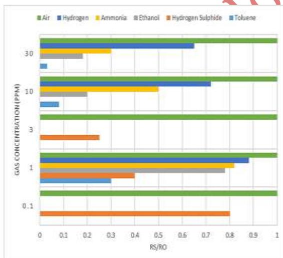
Fig. 2: TGS2602's sensitivity to various gases ( $R_s/R_o$ ).
