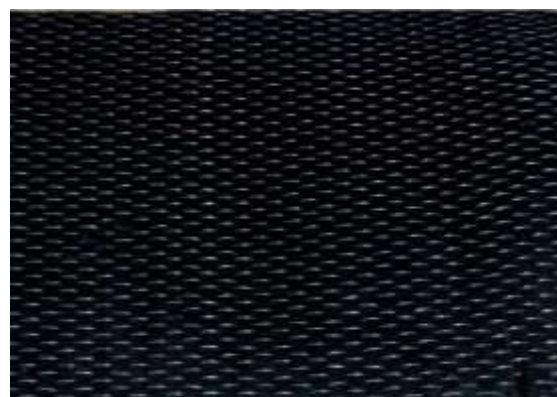
Figure 1: Carbon fabric bundles of filament tie together by polyester
