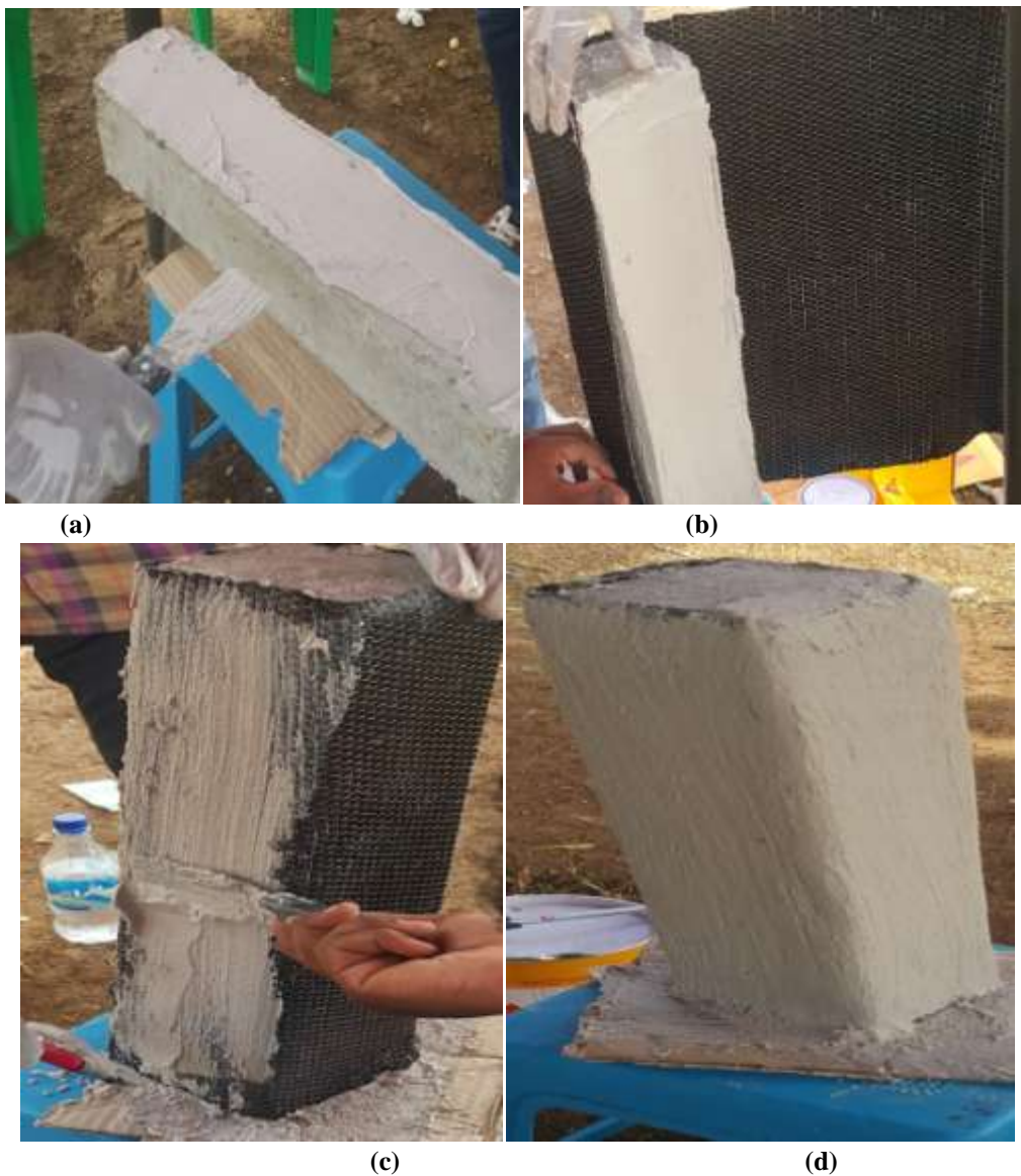
Fig 5: Coated and painted concrete with carbon fabric
