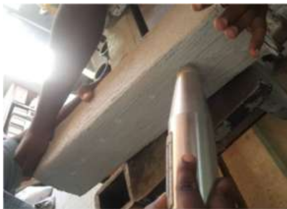
Fig: Hammer test for carbon fabric coated concrete
