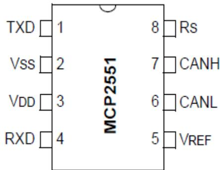
Fig 2. Pin diagram of MCP2551
