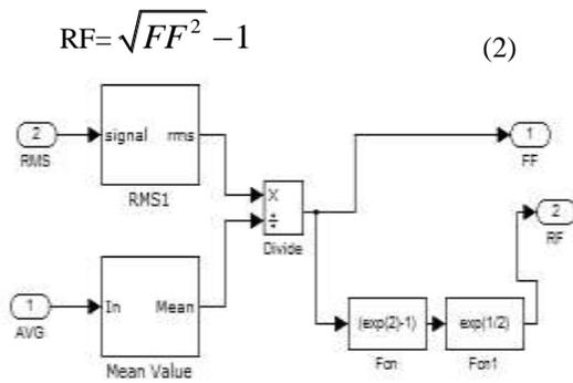
Fig 15: Calculation of Form Factor and Ripple Factor
