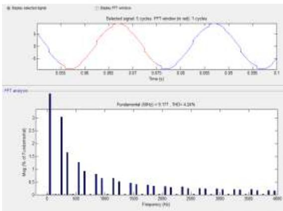
Fig 11: FFT of the 24- Pulse Converter
