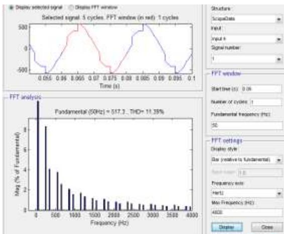
Fig 7: FFT of 18-Pulse Converter
