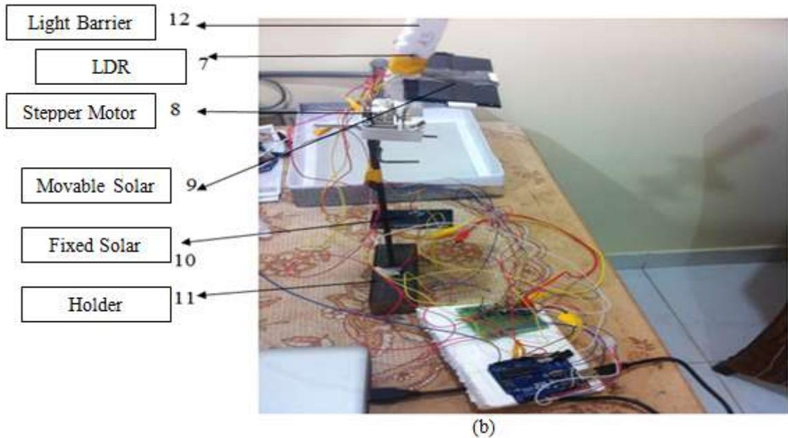
Fig 2: (a). (b). The proposed Setup of the Proposed Solar Tracker
