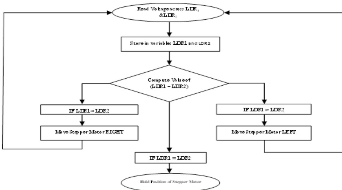
Fig1: Flowchart of the Solar Tracker
