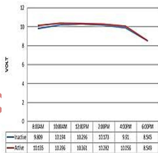
Fig10. Voltages generated from the 3 W Cell
