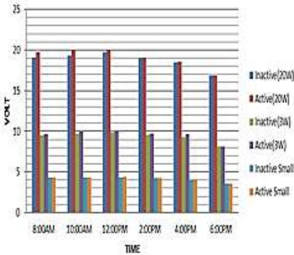
Fig7: Test5. Voltage generated from the three cells at different time in a day
