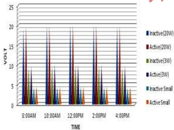
Fig3: Test1: Output voltages generated from the three cells at different time in a day
