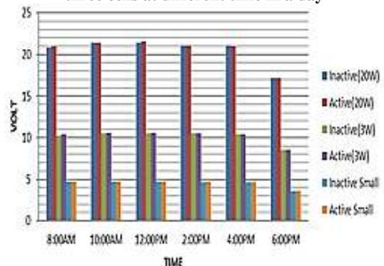
Fig5: Test3: Output voltages generated from the three cells at different time in a day
