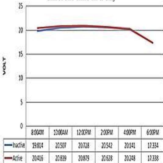
Fig8. Voltages generated from the 20 W Cells
