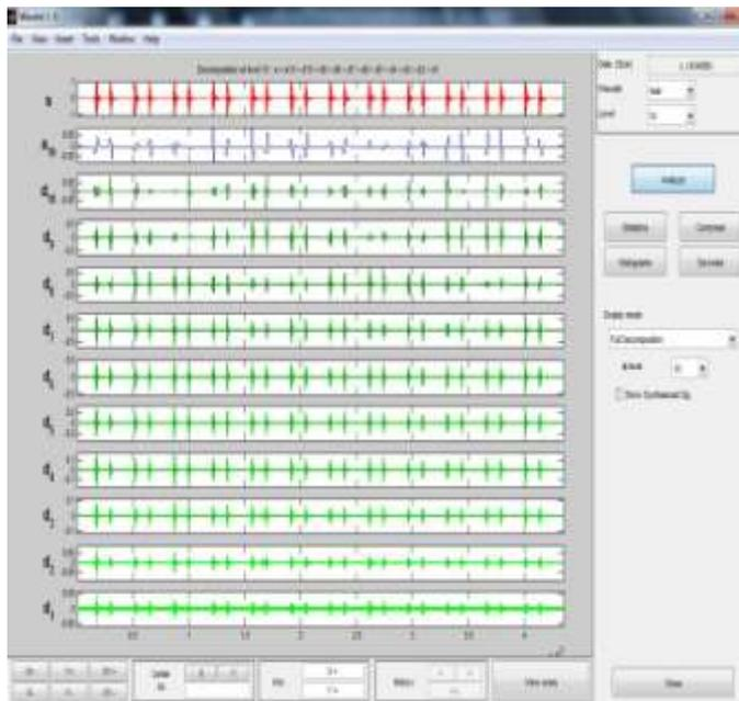
**Fig. 13 Wavelet Decomposition of Normal.wav using Haar Wavelets at level 10**
