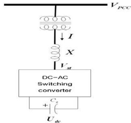
Fig.5.1 single-line diagram of var generator by rotating a voltage-sourced switching converter
