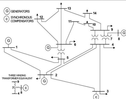
**Fig.6.1: Single line diagram of IEEE-14 Bus system**
