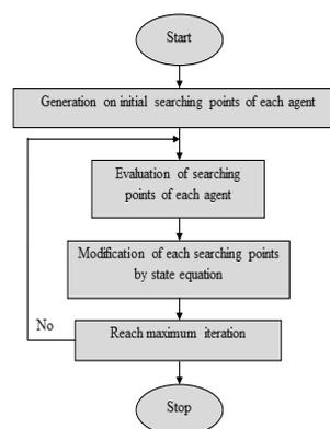
Fig.4.1.Flow chart of PSO algorithm
