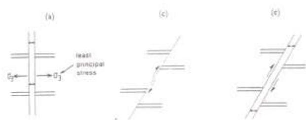
**Figure 6: The basic types of joints (after MacClay 1987)**
