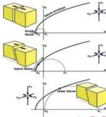
Figure 7 Tension shear joints
