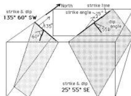
**Figure 5: Fracture patterns developed in joints and measurement of the angles of joint**
