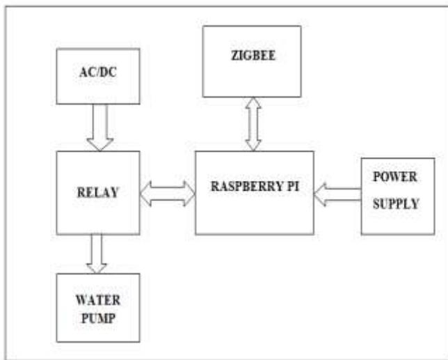
Figure 1: Block Diagram of the Master side of the System
