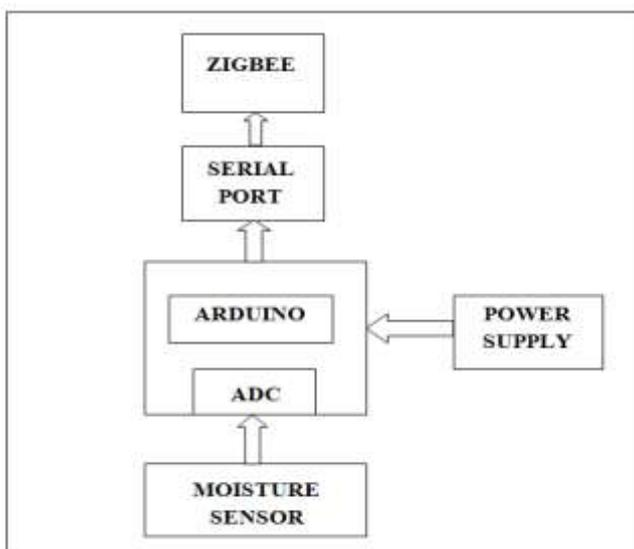
Figure 2: Block Diagram of the Slave side of the System
