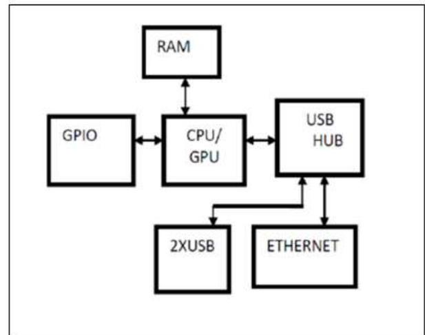
Figure 3: Block Diagram of Raspberry Pi model B
