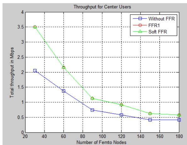
**Fig.6 Sum Throughput of Center users inside a macro cell for varying number of HeNB**
