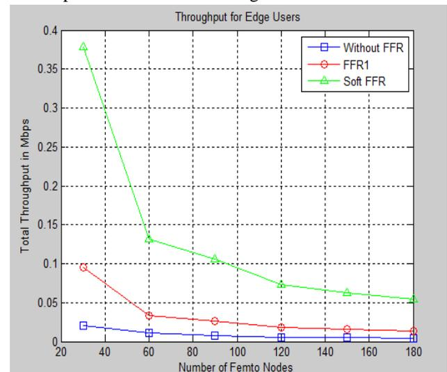
**Fig.5 Sum Throughput of Edge users inside a macro cell for varying number of HeNB**
