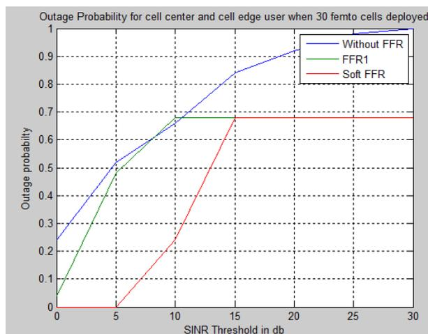
**Fig. 7 Outage Probability for cell center and edge users for 30 femto node**
