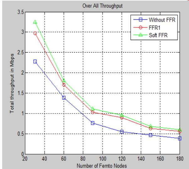
**Fig.4 Sum Throughput of all the users inside a macro cell for varying number of HeNB**
