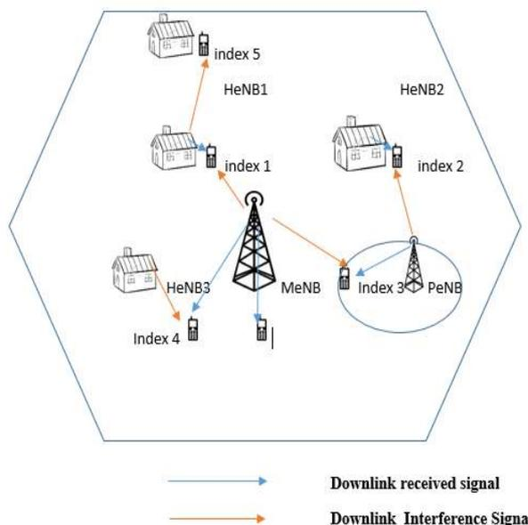
**Fig.1 Heterogeneous Wireless Network with Interference scenario**
