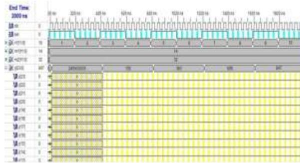
Figure 5.6: Test Bench Waveform of 12 Bit Row Processor in Xilinx
