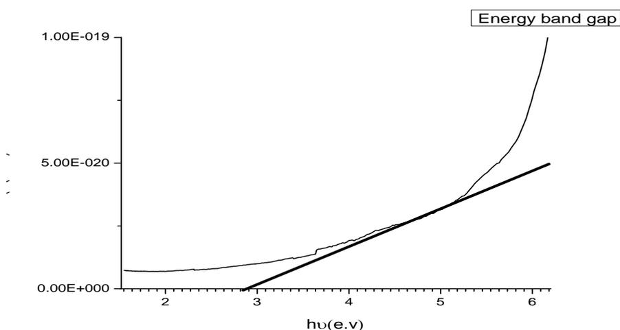
Fig (9): UV-vis spectrum and  $(\alpha h\nu)^2 - h\nu$  curve of the  $Co_3O_4$  Nanoparticles
