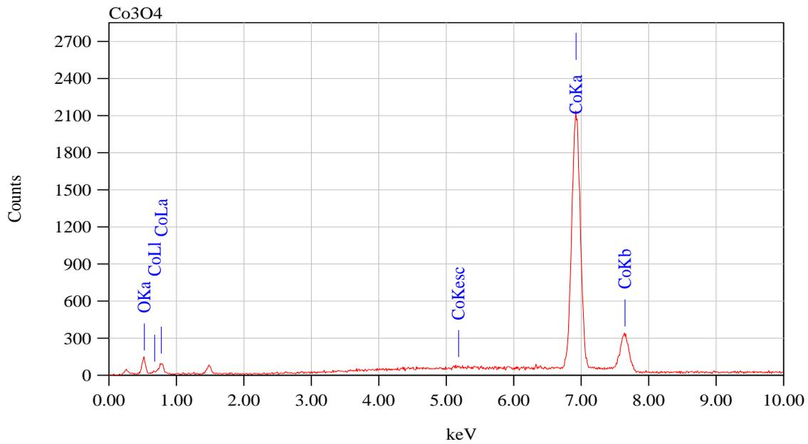
Fig (2): EDX spectrum of  $Co_3O_4$
