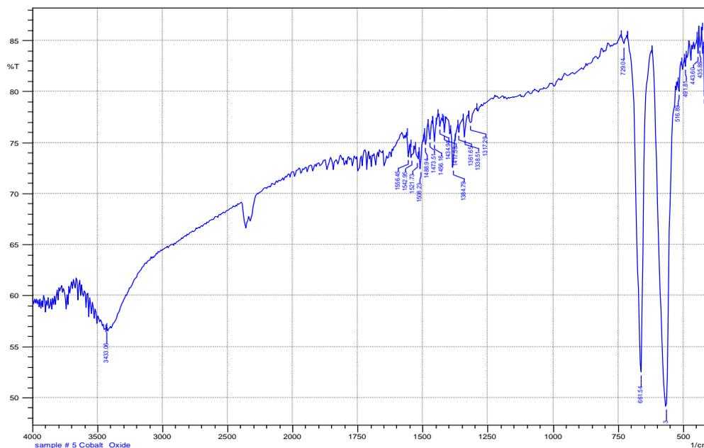
**Fig (1): FT-IR spectrum of  $Co_3O_4$**
