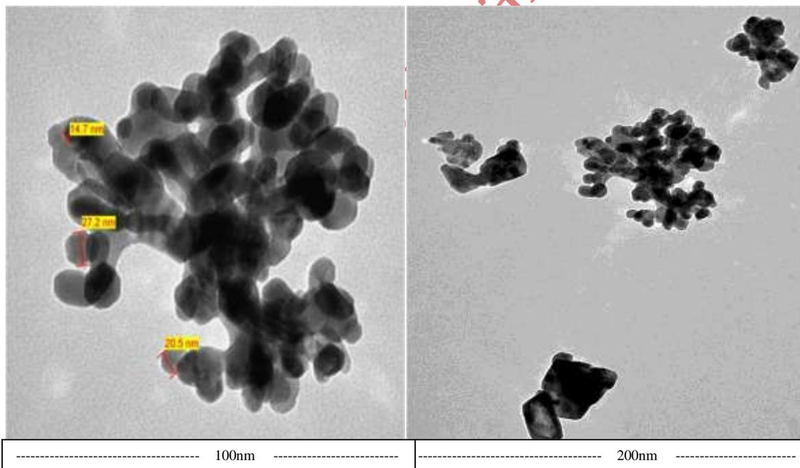
Fig (5): The particle size and nanographs of  $Co_3O_4$  NPs in room temperature measured by using TEM (magnification=300000, model JEM 1400, operating at 90 kV, for 1h at room temperature)
