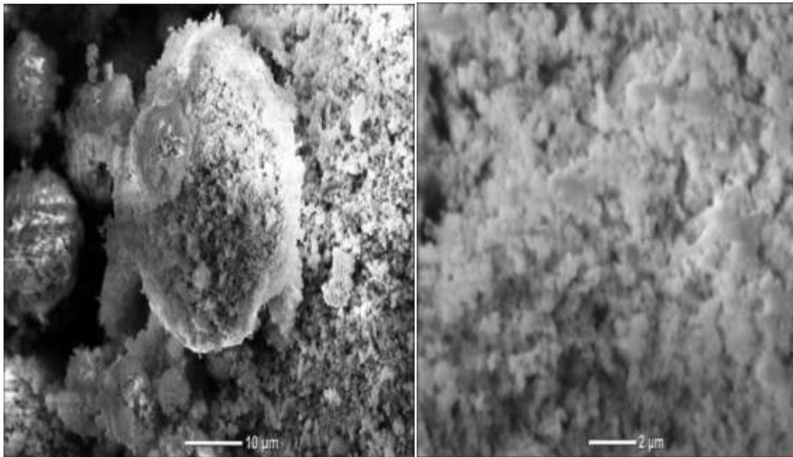
Fig (4): Show the SEM images of  $Co_3O_4$  NPs (a) in  $10 \mu m$  and (b) in  $2 \mu m$  and
