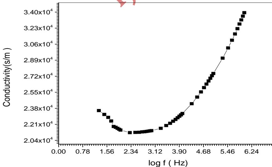
Fig (7): The conductivity of  $Co_3O_4$  NPs.
