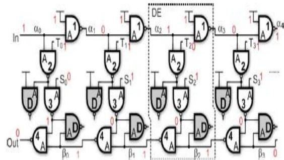
Fig.1 Inverting Glitch Free Circuit of NAND Gate
