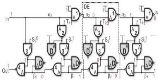
Fig.2 Non Inverting Glitch Free Circuit of NAND Gate.
