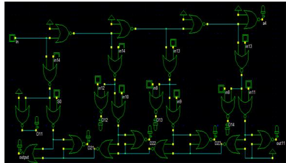
Fig.3 Inverting Circuit using NOR gate.
