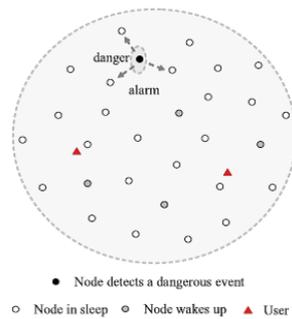
**Fig. 1. Dangerous incident monitoring with a WSN**
