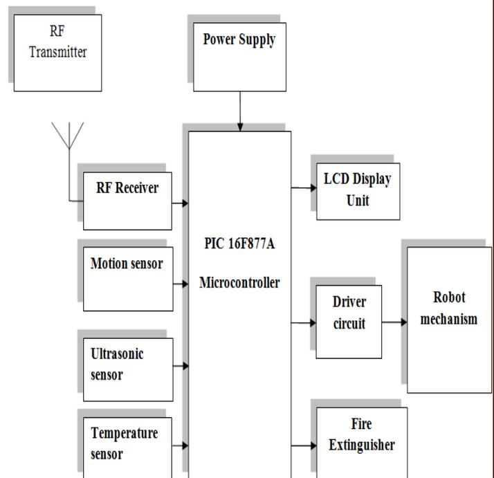
Fig1. Block Diagram representation of advanced DAS system
