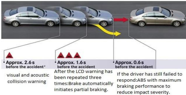
**Fig7. Vehicle Collision Avoidance**
