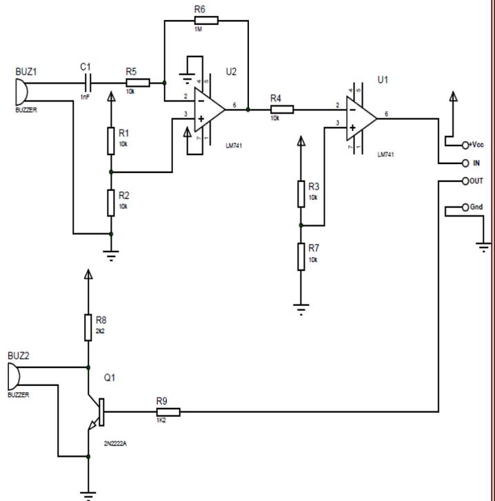
**Fig3. Ultrasonic sensor**
