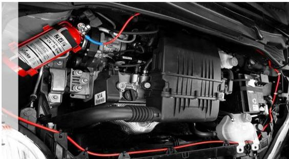
**Fig8. Engine Fire Extinguisher**
