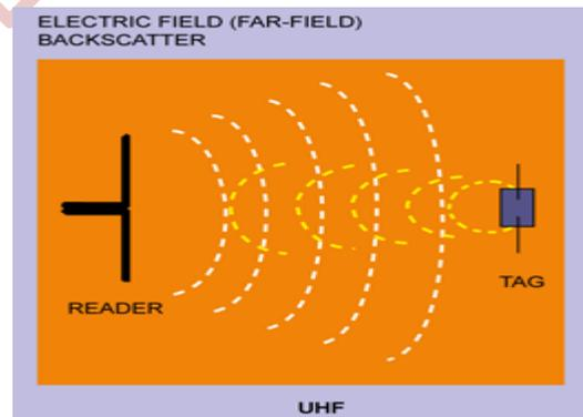
**Fig10. Radio Frequency Identification**
