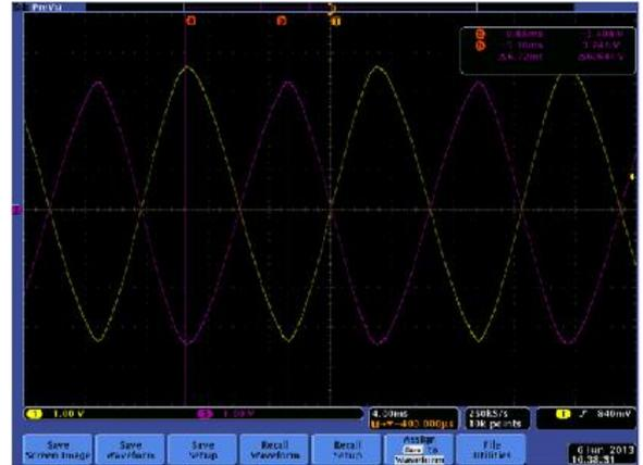
**Fig. 8: Sine Wave Filter Output**
