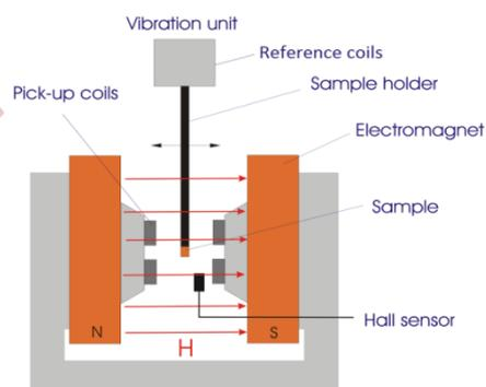
**Fig.1: Schematic diagram of a vibrating sample magnetometer**
