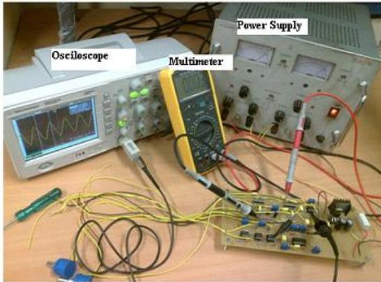
**Fig. 6: Hardware circuit design with some measurement devices and power supply**
