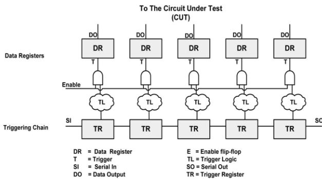
Fig 6. Architecture of Selective Trigger Scan-Chain.
