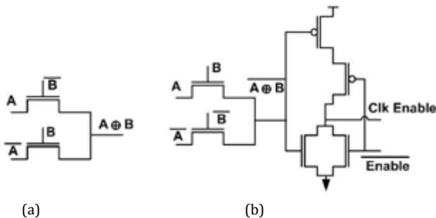
Fig 8. (a) A two-transistor XOR. (b) The structure used for implementing the Clk Enable signal of the DR flip-flops.
