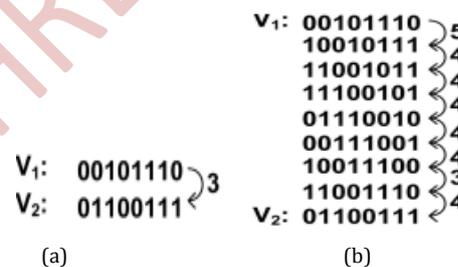
Fig 5. (a) Necessary transitions between two consecutive test vectors(three transitions).
