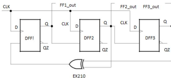
Fig 1. Block Diagram of Linear Feedback Shift Register
