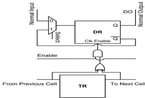
Fig 7.Scan Cell Structure for Selective Trigger Architecture
