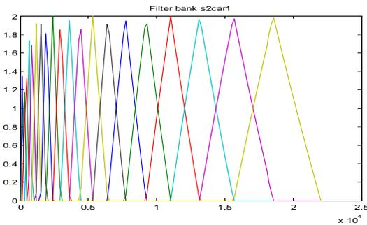
**MEL-SPACED FILTER BANK (K =20) PLOT FOR ORIGINAL CAR NOISE IN MATLAB**
