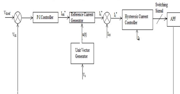
**Fig: 4 Basic circuit of active power filter**
