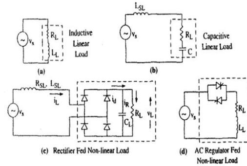
**Fig: 3 Different types of loads**
