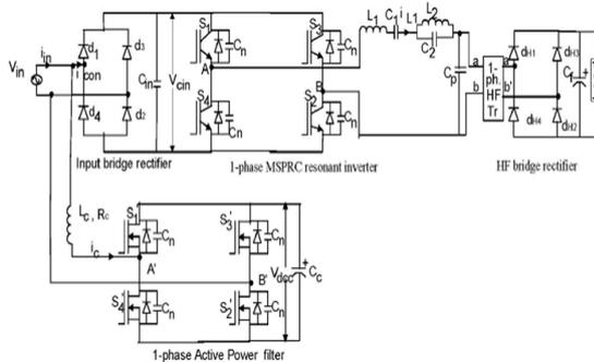
**Fig:2 Single phase ac-to-dc resonant converter with ACF**
