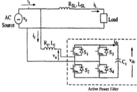
**Fig: 1 Basic circuit of Active Power Filter**
