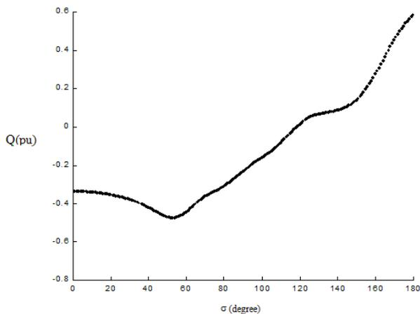
**Figure 10. The modifications of reactive power for several conduction angles.**
