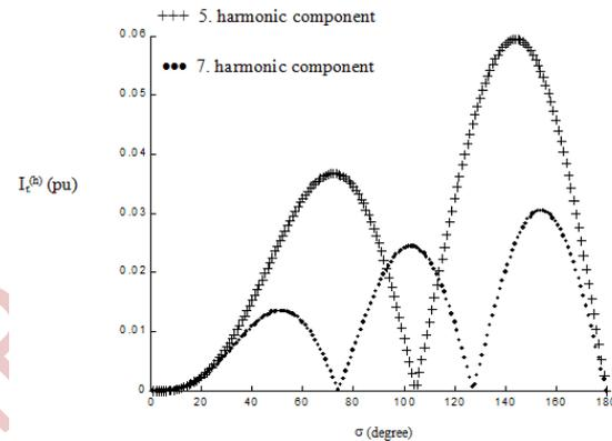
**Figure 8. Harmonic current parts versus conduction angle ( $\sigma$ ).**
