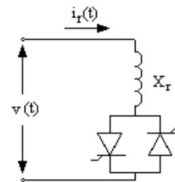
Figure 1. The main components of a TCR
