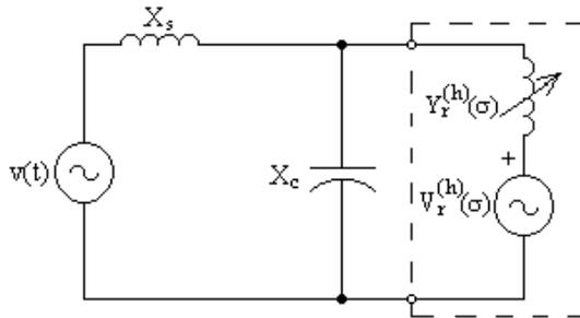
**Figure 4. Variable voltage supply and admittance model for a TCR.**
