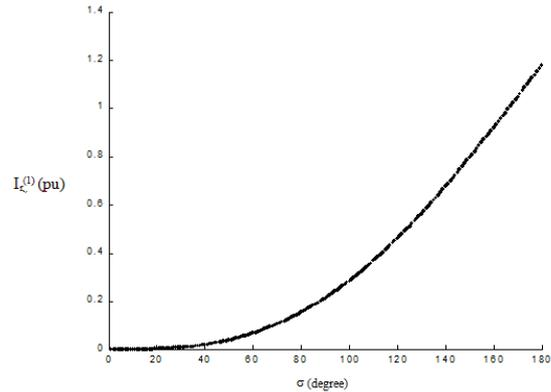
**Figure 7. Basic current aspect versus conduction angle ( $\sigma$ ).**
