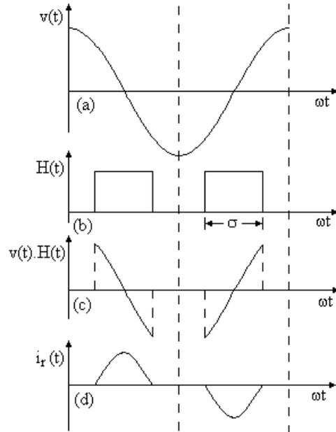
**Figure 3. Voltage and current waveforms of TCR.**
