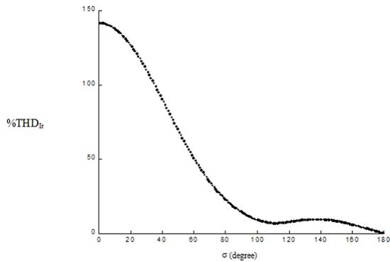
**Figure 9. THD<sub>r</sub> versus conduction angle (σ).**
