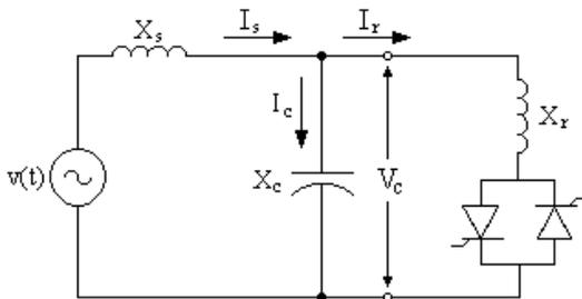
**Figure 2. Fixed capacitor-thyristor controlled reactor static VAR compensator.**
