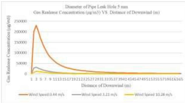
**Figure 1 Gas Concentration at 5 mm Pipe Leak Hole Diameter**
