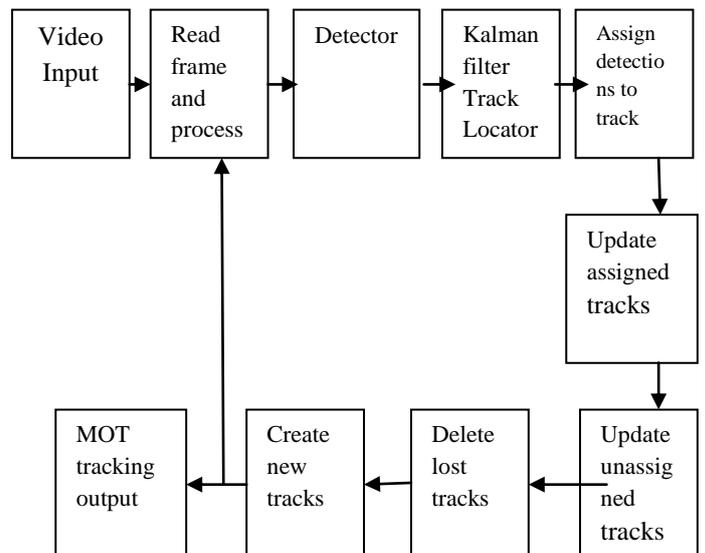
Create new tracks block Create new tracks from unassigned detections. MOT tracking output block displays the results of multiple object tracking draws a bounding box and label ID for each track on the video frame.
