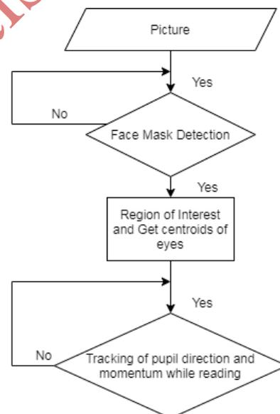
Figure 2: Block Diagram for Eye Ball Detection, Explanation, and final output,
