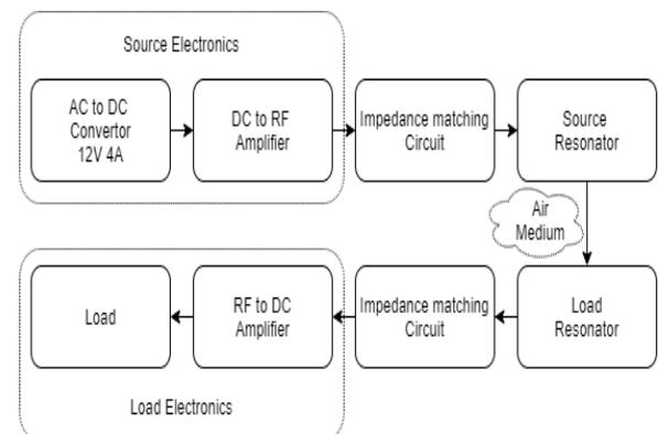
Fig[F]: Block diagram of working principle of WPT
