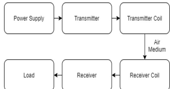
[Fig: A:] Mutual inductance based wireless power transfer Method
