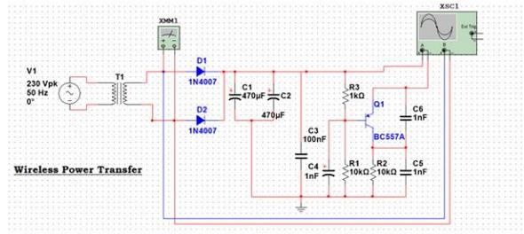
Fig. [G] Simulation on Multisim
