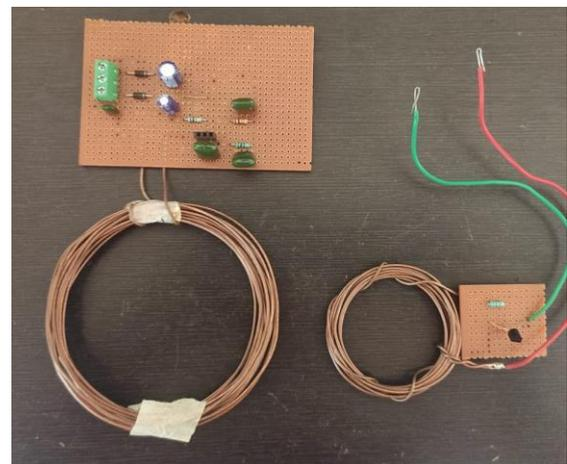
[Fig: B:] Mutual inductance based wireless power transfer Circuit
