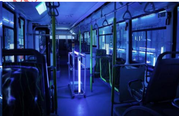
Fig. 30 - Bus disinfection through UV lights. A way to fight Coronavirus in Shanghai. Credits: https://www.sustainable-bus.com/news/bus-disinfection-through-uv-lights-a-way-to-fight-
