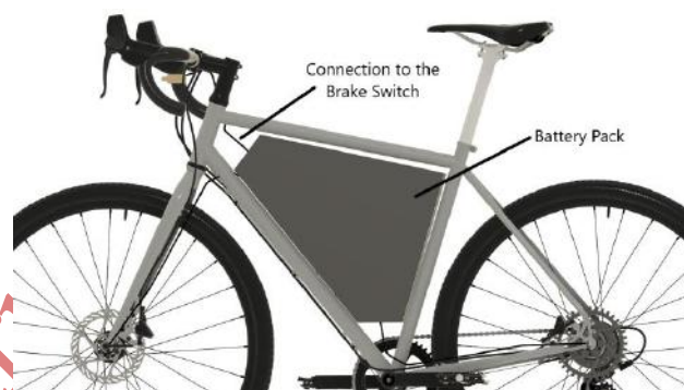
Fig.2. CAD model of the Battery Casing
