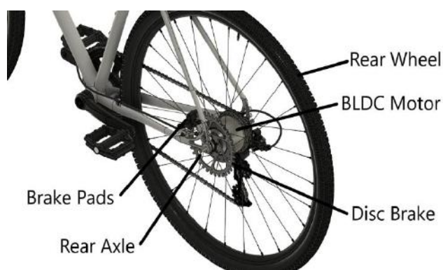
Fig.1. CAD model of the rear wheel
