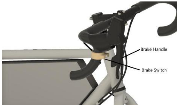
Fig.3. CAD model of the Auto-switch
