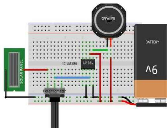
Fig 6: Breadboard diagram of LiFi Receiver
