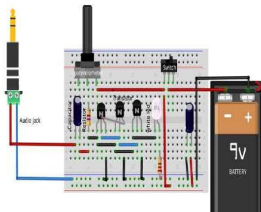
Fig 5: Breadboard diagram of LiFi Transmitter
