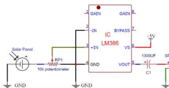
Fig 8: Circuit diagram of LiFi Receiver
