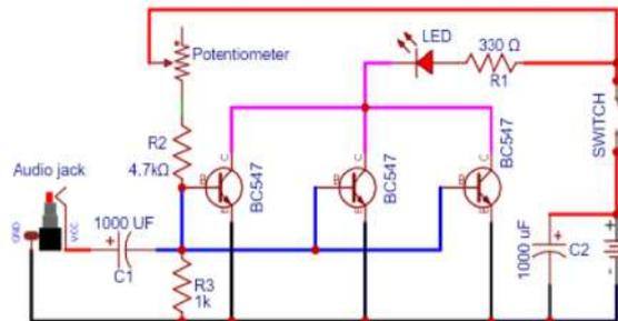
Fig 7: Circuit diagram of LiFi Transmitter
