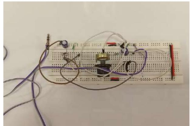
Fig 9: Practical implementation of LiFi Transmitter
