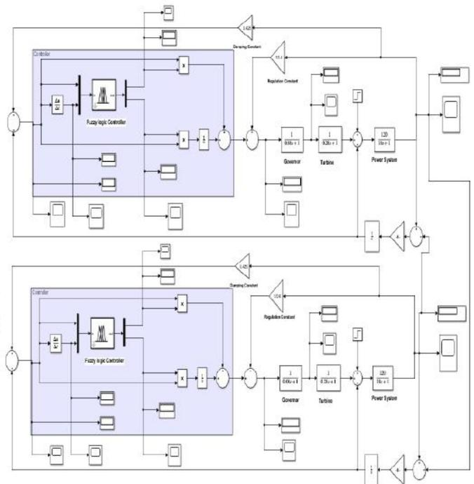
Fig 4 Simulink model of LFC using ANFIS controller
