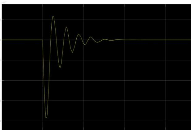
Fig 3 Change in frequency ( $\Delta f$ ) response for ANN-PI controller.
