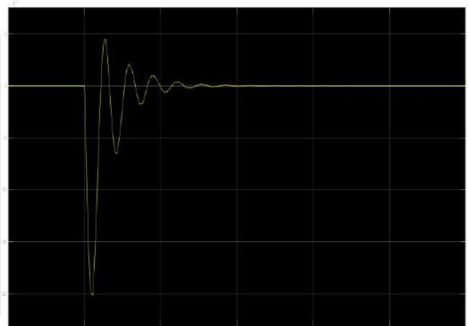
Fig 5 Change in frequency ( $\Delta f$ ) response for ANFIS controller.
