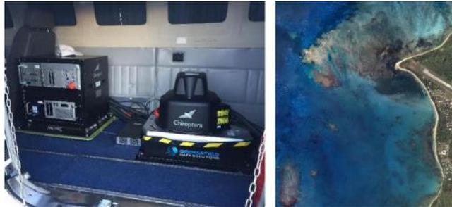
[FIG:A] Mapping underwater terrain with bathymetric LiDAR Technology
