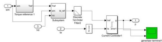
Fig : MPPT for Wind Generator
