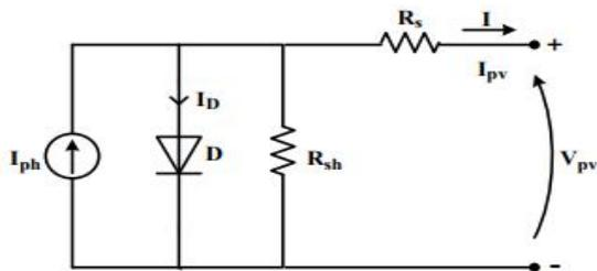
Fig1: The equivalent circuit of a PV array.
