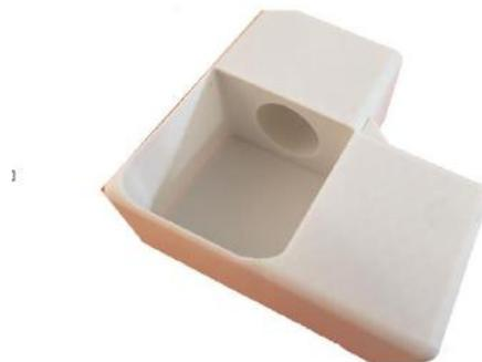
We have made a special 3D Printed holder which combines all the components like camera, laser and the sample container into a single unit. This is a L shaped block which can hold the camera on one side and the laser on the other side so that both of them point directly to the water sample container at the angle of 90 degree.
