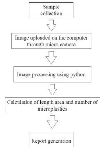
Our Solution is handy, easy to use, and built on practicability. The simple mechanism of a microcamera and image processing tools/code enable us to get accurate data at a domestic level. The code implemented uses technology to ensure that the margin of error remains minimal.
