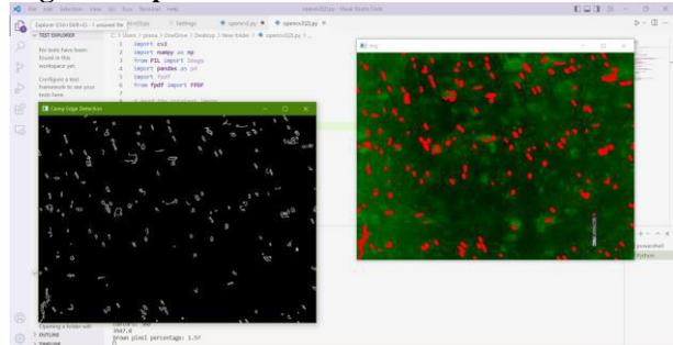
On the left, we can see the contours detected from the image. Right, we mark the detected microplastic on the original image with red.
