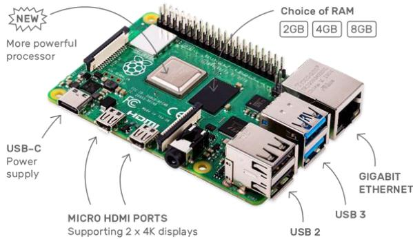
I am using the Raspberry Pi4 as the main computer of the robot . It is the latest and the fastest model available for making smart computer based projects. It helps in making the prototype compact and really portable
