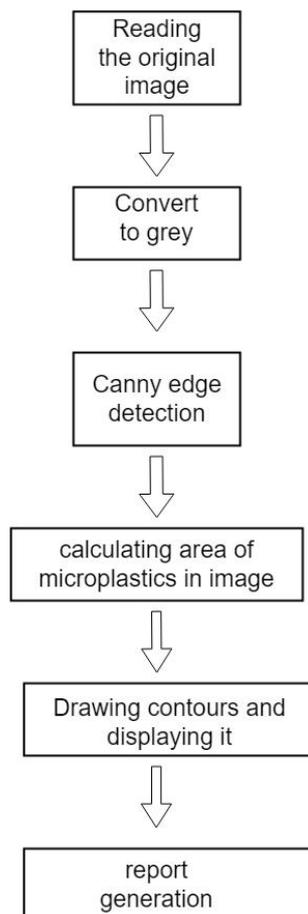
CV2 is a python library known for its code readability and simplicity. We use CV2 for converting image to grey and specifying thresholds for canny edge detection
