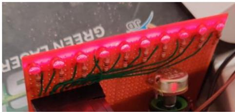
We have made our own LDR sensor array to make it compact. It takes very less space as there is only a 1cm gap between the sensors. The full array covers the area of 10 cm which is more than enough to sense and differentiate between urination and defecation.
