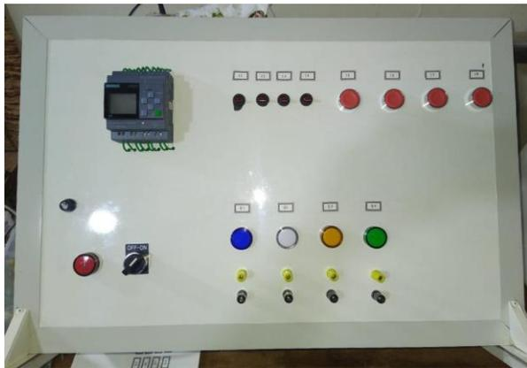
Fig.4: Programmable logic control panel
