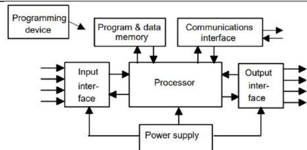
Fig.3: Block diagram for PLC panel. [7]
