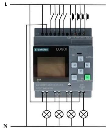
Fig.2: Wiring diagram for PLC panel.
