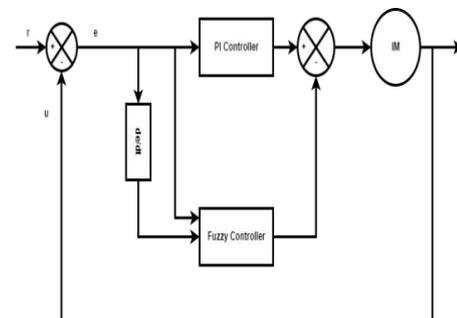
Fig.5 Block Diagram of Fuzzy Tuned PI Controller
