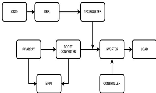
Fig.1(a) Multi-Mode Grid Linked Solar PV
