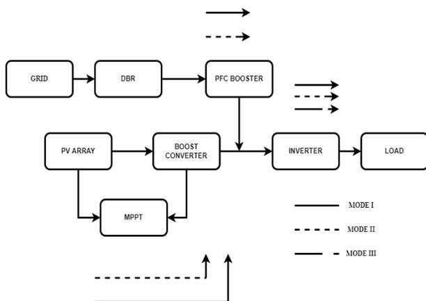
Fig.1(b) Different Power Flow Mode
