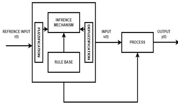
Fig.2 Block Diagram of Fuzzy Controller
