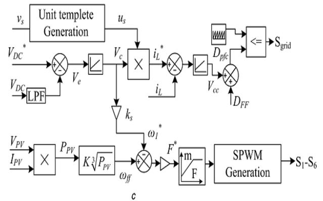
Fig.1(c) Control Scheme of Grid Connected Solar PV
