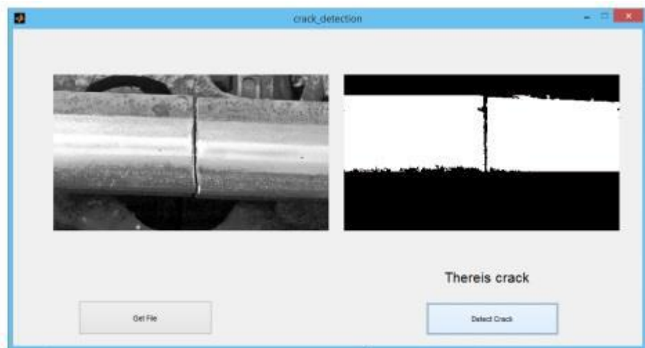
Figure 7: Crack Present is detected
