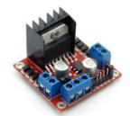
L298 module is a high power efficient motor driver circuit which can give high current to all the high torque DC Motors in the robot circuit.
