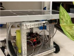
We have used tetrix aluminum channels to design the mechanical structure of the chassis. It has 2 tetrix DC Geared motors in the driving mechanism.
