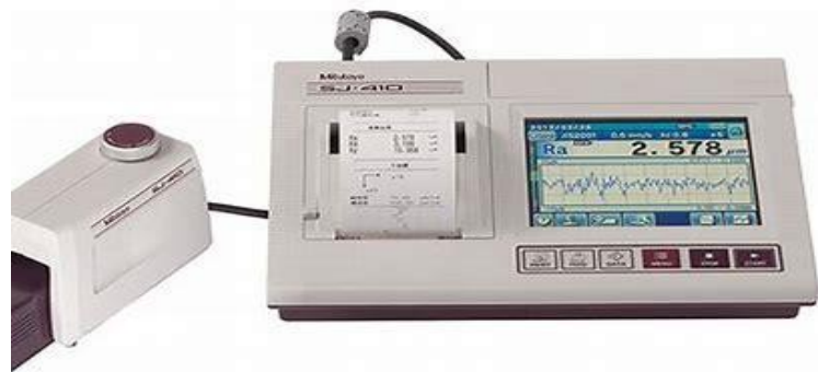
Figure 3.2: MITUTOYO 178-602 Surface Roughness tester measuring the roughness of surface machined by milling macheni
