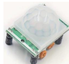
Fig. 6: PIR motion sensor.
