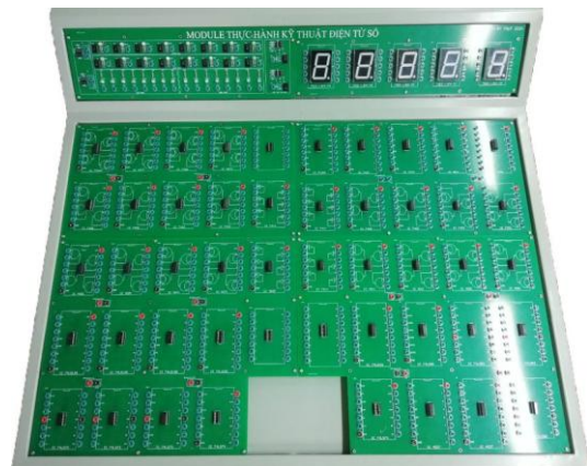
Fig. 12: The image of the multi-purpose practice table for the digital electronics subject has been completed
