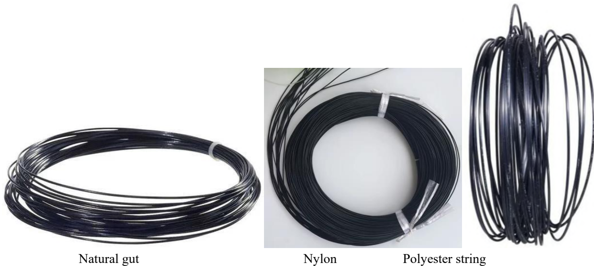
Figure 1. Tennis racket string materials typically employed in practice and incorporated in the present experimental study.
