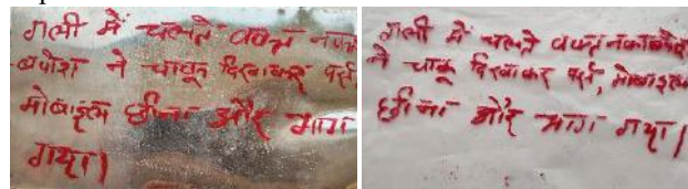
Figure.2 Smooth line formation on non-porous surface (aluminium, plastic)
