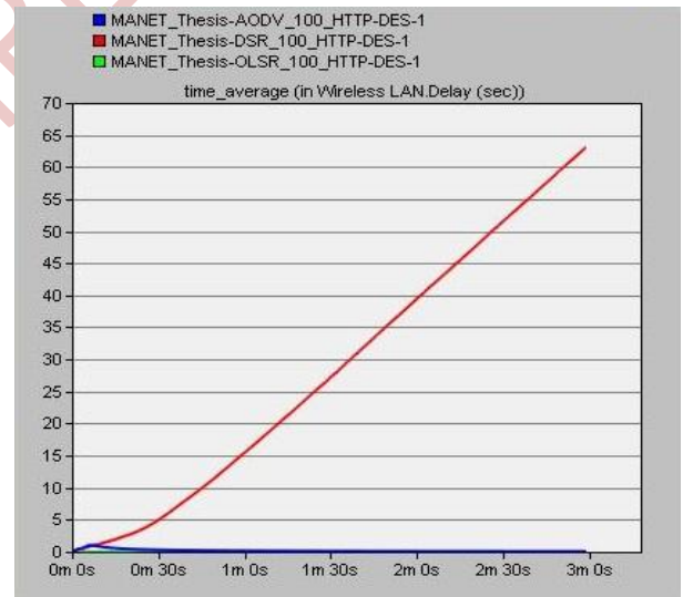
Fig 3: Delay comparison in three routing protocols for 40 nodes
