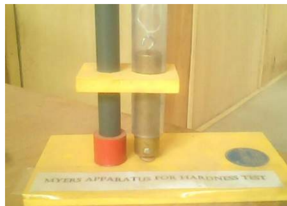
Plate 2: Myer's Apparatus for Hardness Test.
