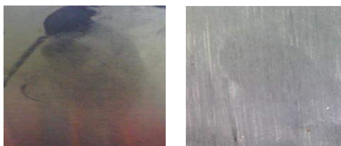
Fig3. objects submerged for 45 days of aluminium samples subjected to SPR white
