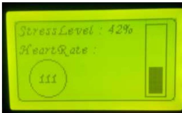
Figure 4. Heart rate and Stress level is displayed on GLCD
