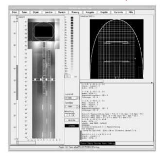
Figure 1. Output generated by the BUT system. Left side: Illumination plan generated by BUT. Right side: Front view of a shaft in a mine.
