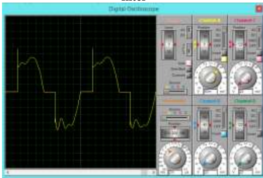
Figure 11 Current waveform after applying C-type filter
