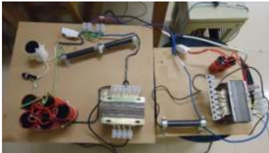
Figure 16 C-type filter for 3rd harmonic (left) and second order high-pass filter for 5th harmonic (right)
